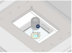
matching adapter ring. Always make sure that the objective adapter ring is screwed in tightly. Afterwards turn on the NanoOne again, the build room door will close automatically.
