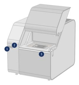
The operating elements of the NanoOne are located on the front left side of the machine. The printing system is started up by actuating the **on/off switch (1)** or switched off after printing. The door is automatically opened or closed by actuating the **door switch (2)**. The machine status is displayed via an **LED status bar (3)** which is illuminated according to the status.
