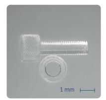
This transparent glass bolt and nut were printed in UpQuartz, resulting in a high-resolution part that is 100% silica glass after a thermal post-treatment.
